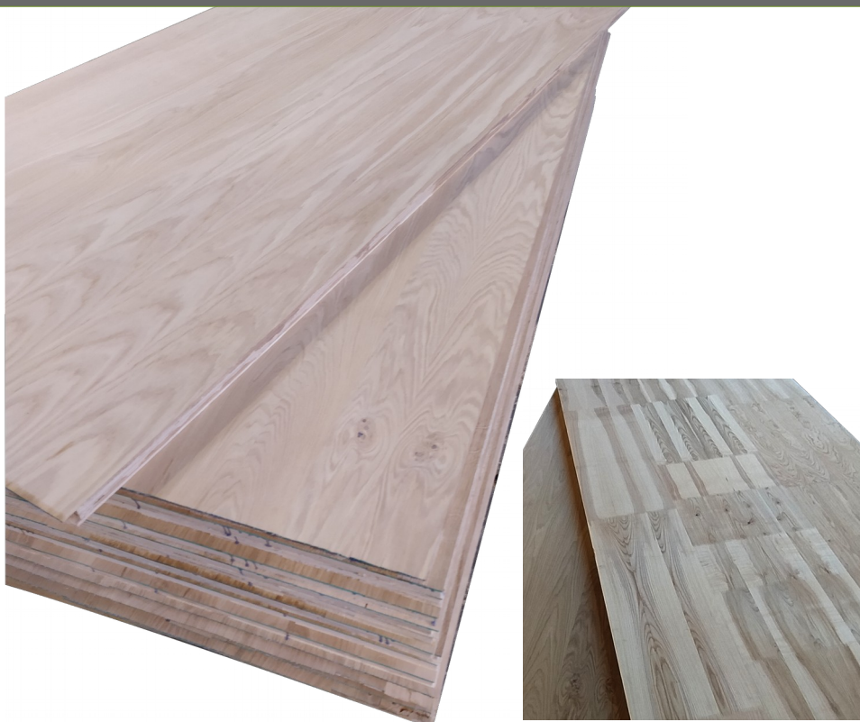
Panneau multi-plis Parements 2,5-3 mm chêne BME Âme Bouleau (importation)
